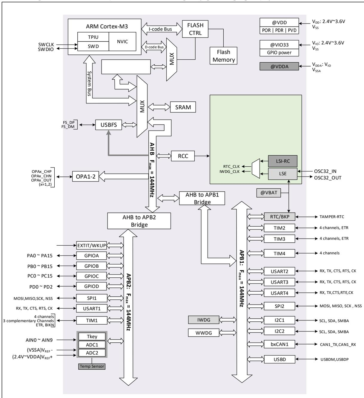
Figure 1-2 CH32V2x (connection/interconnection/high capacity general-purpose) system architecture
