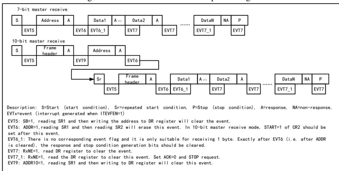
When the master device ends sending data, it will actively send an end event, i.e. set the STOP bit, and the I2C will switch to slave mode. In receive mode, the master device needs to NAK at the answer position of the last data bit, and after receiving NACK, the slave device releases control of the SCL and SDA lines; the master device can then send a stop/restart condition. Note that the I2C module will automatically switch to slave mode after the stop condition is generated.
