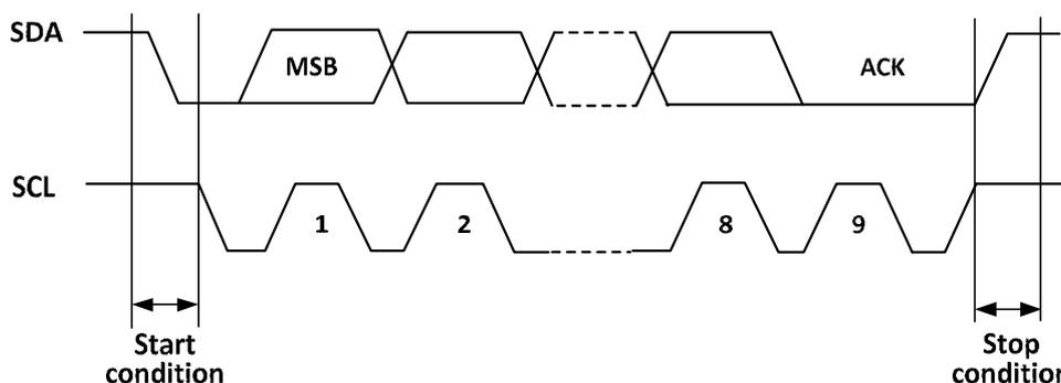
For normal use, the correct clock must be input to I2C. In the standard mode, the minimum input clock is 2MHz, while the minimum input clock is 4MHz in the fast mode.
