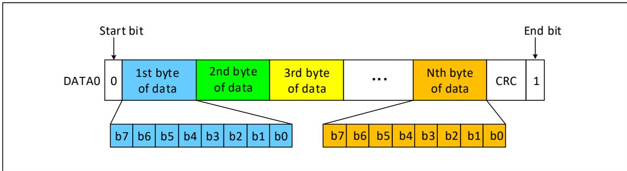
Figure 28-10 SD card 4 bus data transfer byte format
