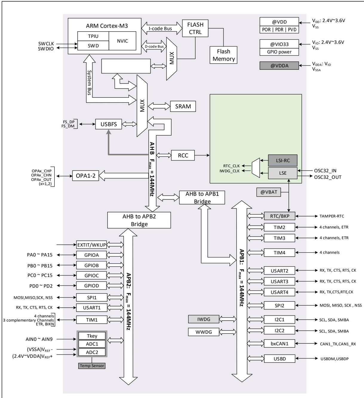
Figure 1-3 CH32F208 (wireless) system architecture
