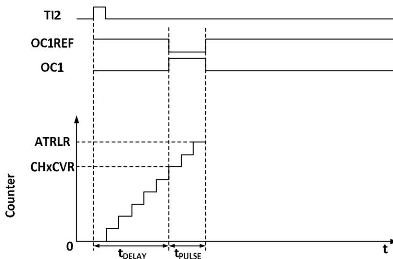
As shown in Figure 15-4, it is necessary to detect the beginning of a rising edge on the TI2 input pin. After delaying  $T_{delay}$ , a positive pulse of length  $T_{pulse}$  will be generated on OC1:
