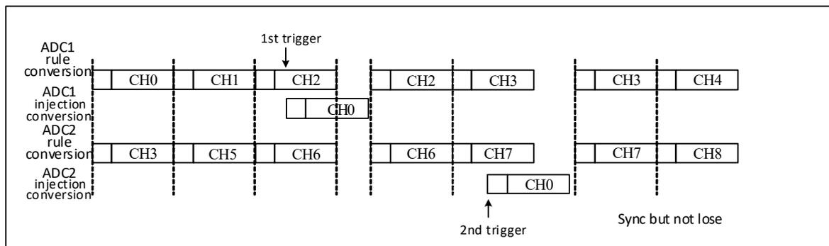
Note: In this mode, the conversion groups of ADC1 and ADC2 should have the same time, or the time of the longer conversion group is less than the trigger time interval.
