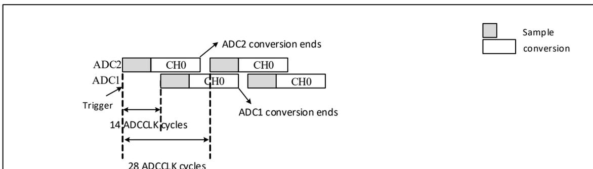
Note: 1. The sampling time should be less than 14 ADC clock cycles, to avoid an overlap with the next conversion;
