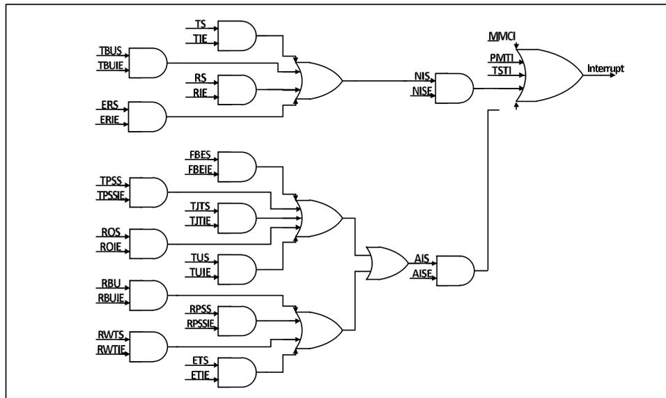
The DMA interrupt is the most important interrupt in the Ethernet transceiver. Generally, user logic needs to rely on interrupts to receive frames, confirm that the frames are sent, or deal with the interrupted transceiver logic in time.
