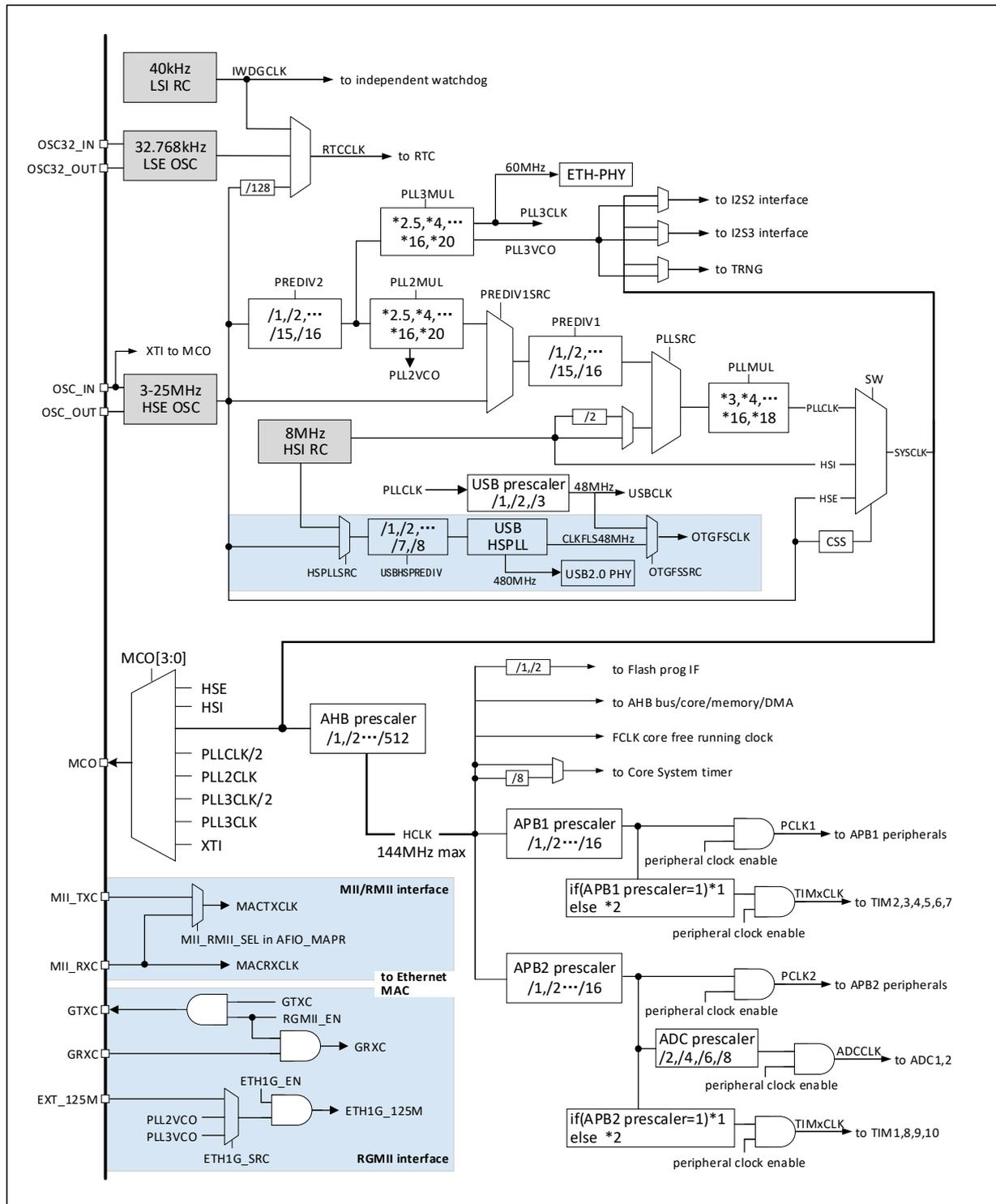
Note: This clock tree structure is applied for CH32F20x\_D8C and CH32V30x\_D8C. When the USB interface is used, the frequency of CPU must be 48MHz or 96MHz or 144MHz. When USBHD high speed function is used, the clock source of USBHSPLL can only be HSE. When system wakes up from sleep state, HSI is automatically switched as system clock frequency.
