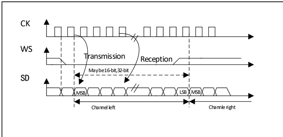
Figure 20-5 Philips protocol waveform (24-bit frame, CPOL=0)
