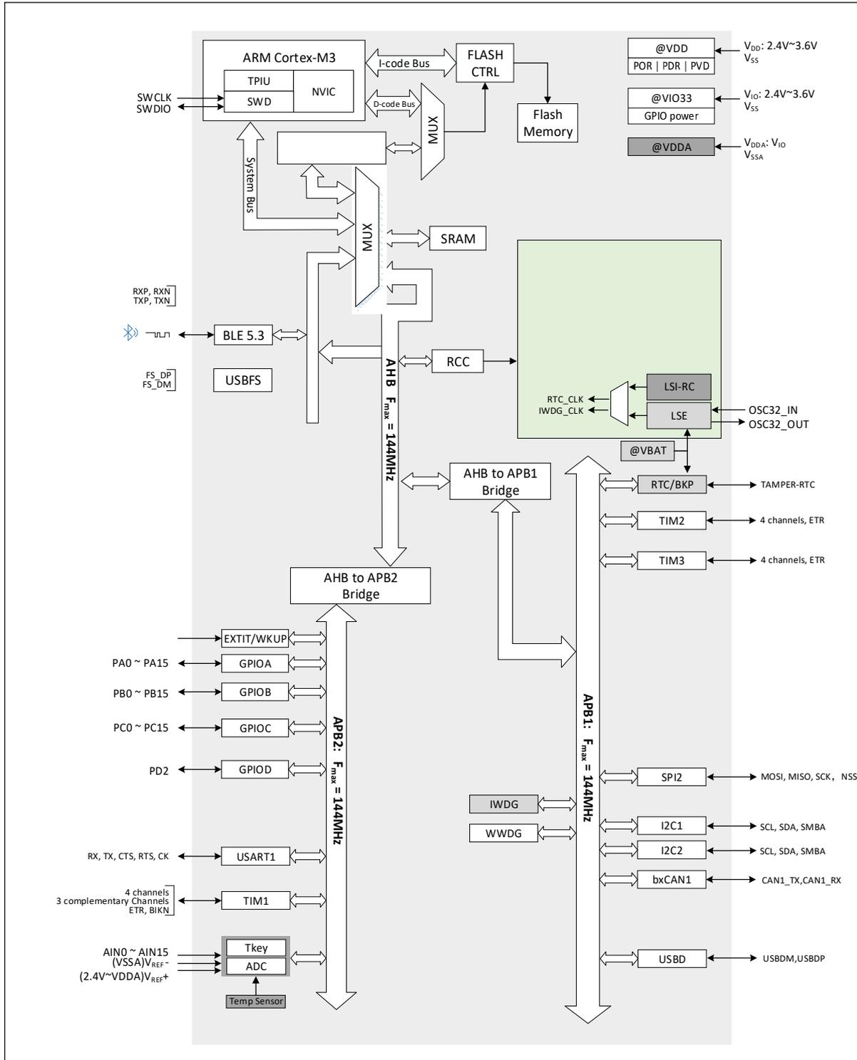
Figure 1-4 CH32V203 system architecture
