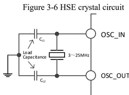
*Note: The load capacitor should be placed as close as possible to the oscillator pins, and the loading capacitance values must be adjusted according to the selected oscillator.*
