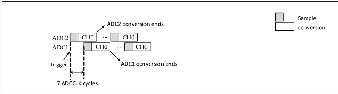
Note: The sampling time should be less than 7 ADC clock cycles, to avoid the overlap between ADC1 and ADC2 sampling phases in the event that they convert the same channel.
