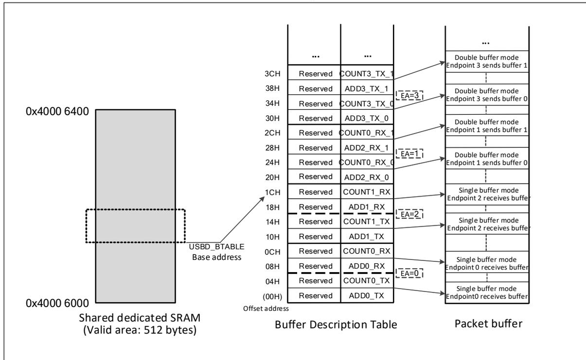
Whether receiving or sending, the packet buffer is used from the bottom. The USB\_D module does not change the contents of other buffers beyond the currently allocated buffer area. If the buffer receives a data packet larger than itself, it will only receive data up to its own size, and the others will be discarded, that is, a so-called buffer overflow exception occurs.
