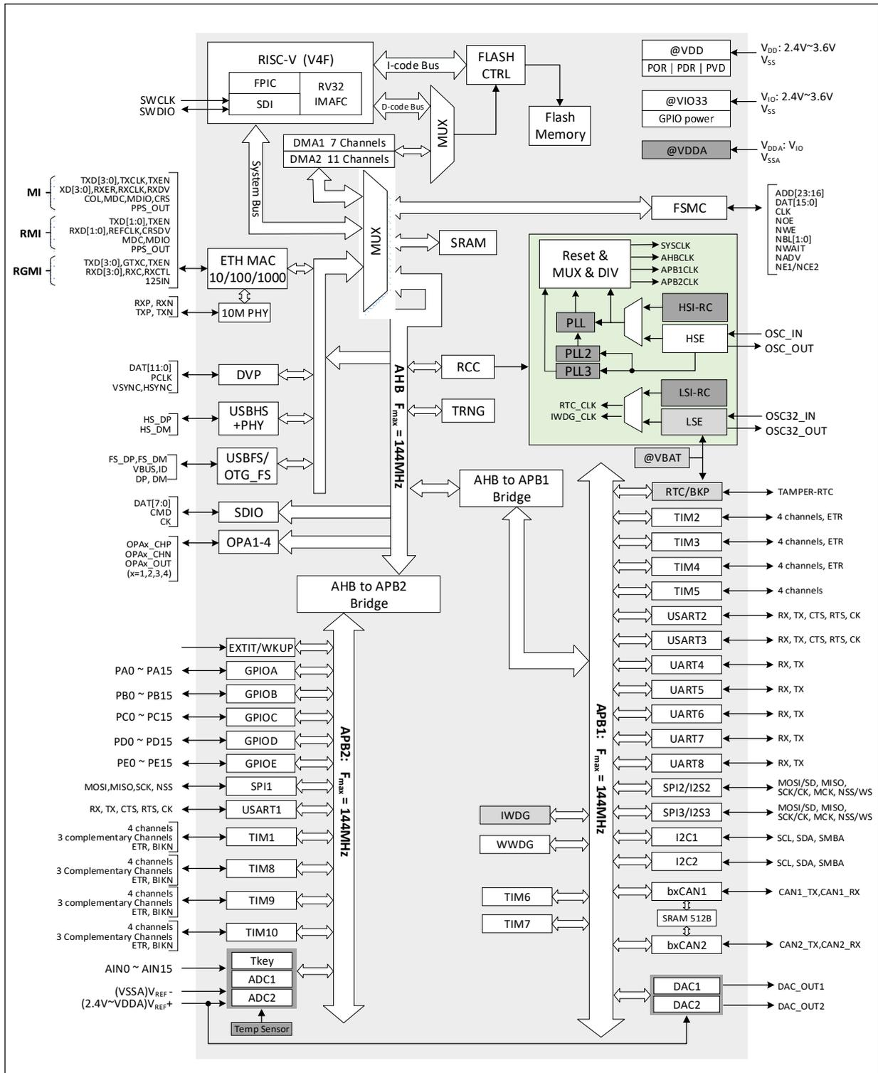
The system is equipped with: Flash access prefetch mechanism to speed up code execution; general DMA controller to reduce CPU burden and improve efficiency; clock tree hierarchical management to reduce the total operating power consumption of peripherals, while being also provided with actions such as data protection mechanism and clock security system protection mechanism to increase system stability.
