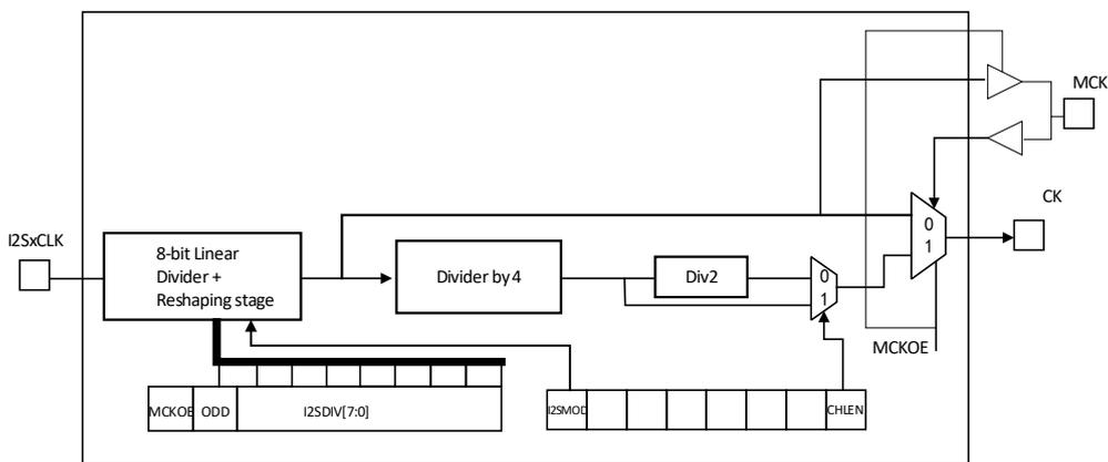
The clock source of I2SxCLK in the figure is the system clock (i.e., the HSI, HSE, or PLL that drives the AHB clock). I2SxCLK can come from SYSCLK, or the PLL3 VCO (2xPLL3CLK) clock, which can be selected by the I2S2SRC and I2S3SRC bits in the RCC\_CFGR2 register. Audio can be sampled at 96KHz, 48KHz, 44.1KHz, 32KHz, 22.05KHz, 16KHz, 11.025KHz, or 8KHz (or any value within this range). To obtain the desired frequency, set the linear divider according to the following formula:
