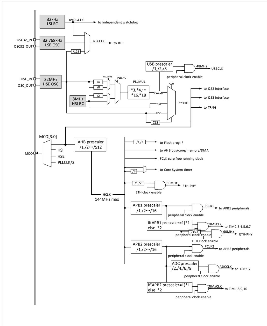
Note: For CH32V203RB, the external crystal or clock (HSE) is 32M. When the external crystal is enabled, no load capacitor is required as it is built in.
