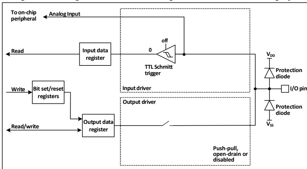
When the analog input is enabled, the output buffer is disconnected and the Schmitt trigger input in the input driver is disabled to prevent consumption on the IO port. The pull-up and pull-down resistors is disabled, and the read input data register is always 0.
