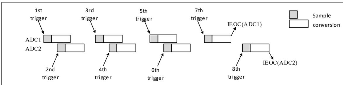
7) Regular simultaneous mode + Injected simultaneous mode
