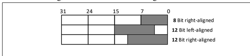
Figure 17-3 Data formats in dual channel mode
