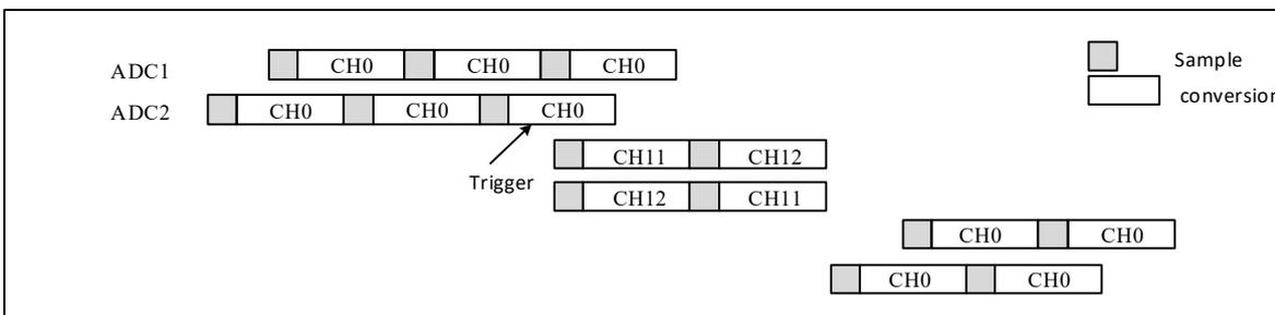
Note: When the ADC clock prescaler is set to 4, the sampling interval is 8 ADC clock cycles followed by 6 ADC clock cycles, instead of 7 ADC clock cycles followed by 7 ADC clock cycles.
