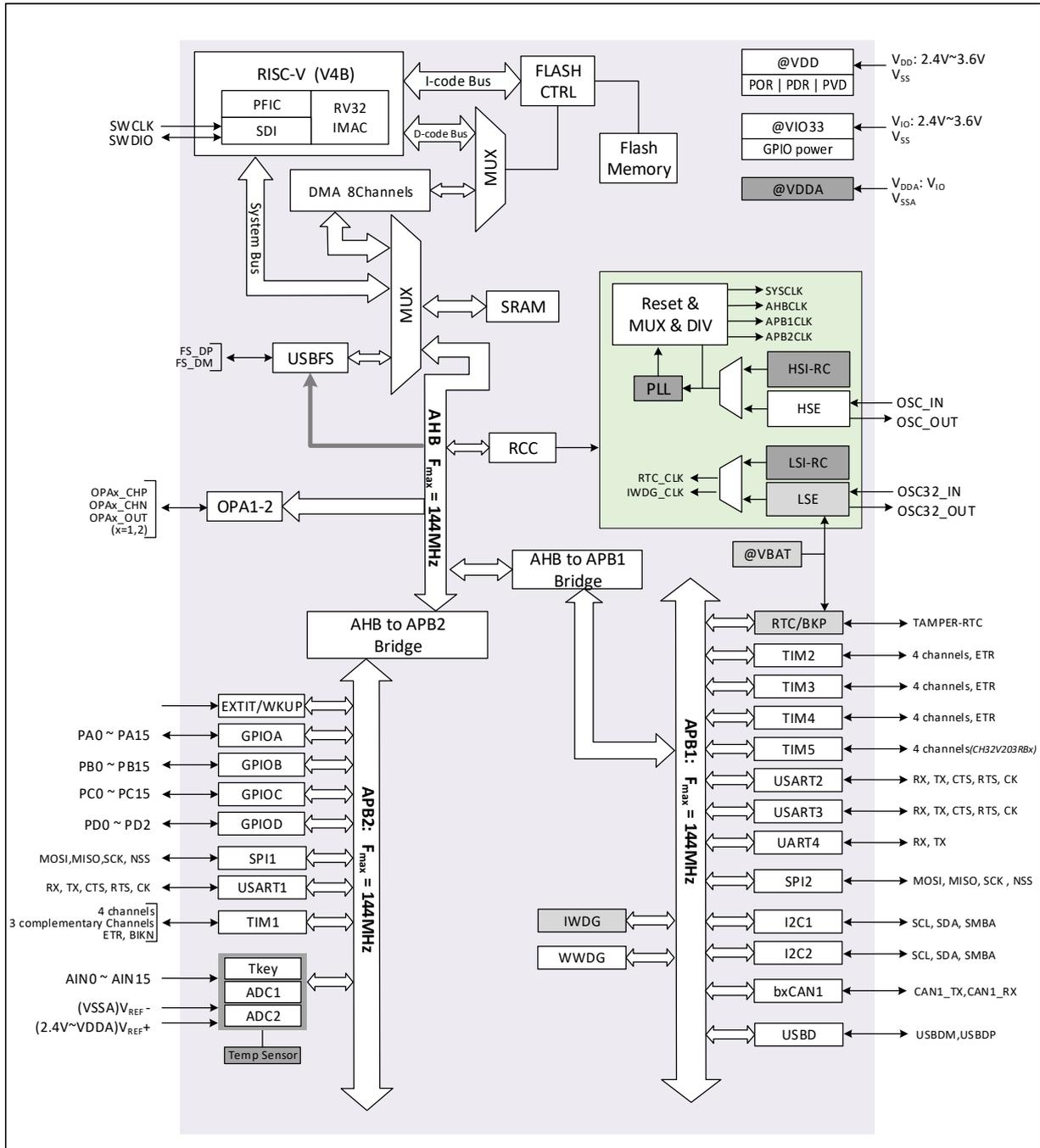
Figure 1-5 CH32V208 system architecture
