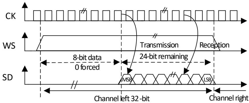
In transmit mode, if you want to send data 0x3478AE, you need to write the register DATAR twice by software or DMA.
