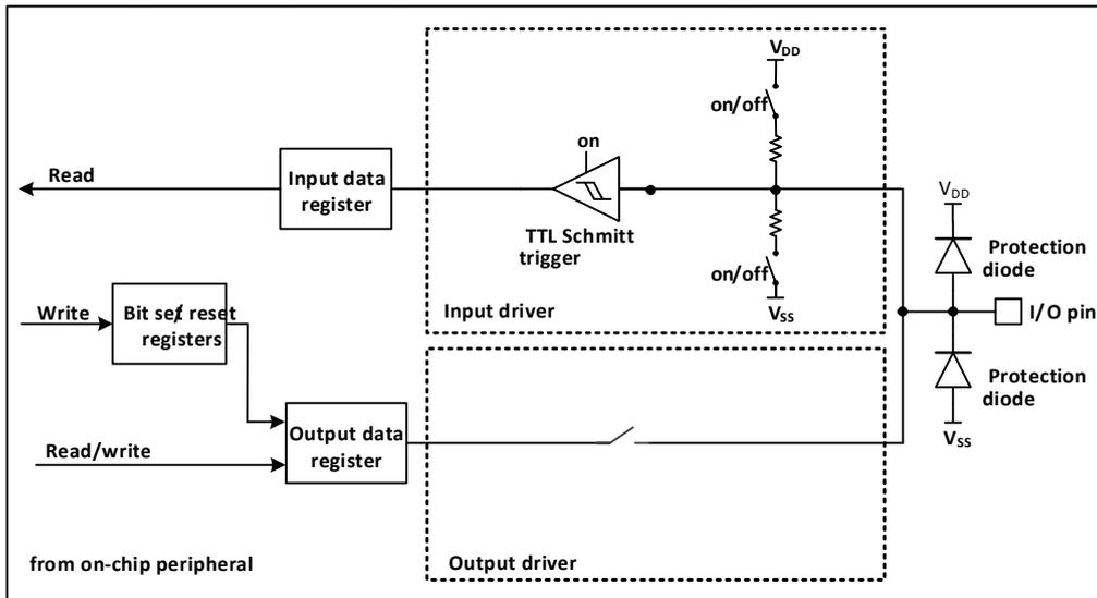
When the IO port is configured as input mode, the output driver is disconnected, the input pull-up and pull-down are optional, and the alternate function and analog input are not connected. The data on each IO port is sampled to the input data register at each APB2 clock, and the corresponding bit of the input data register is read to obtain the level state of the corresponding pin.
