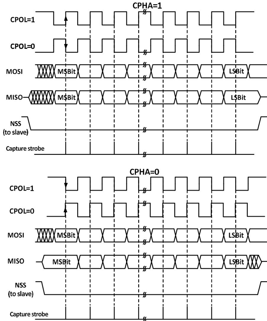
The host and device need to be set to the same SPI mode, and the SPE bit needs to be cleared before configuring the SPI mode. The DEF bit can decide whether the single data length of SP is 8 bits or 16 bits. LSBFIRST can control whether a single data word is big-endian or little-endian.
