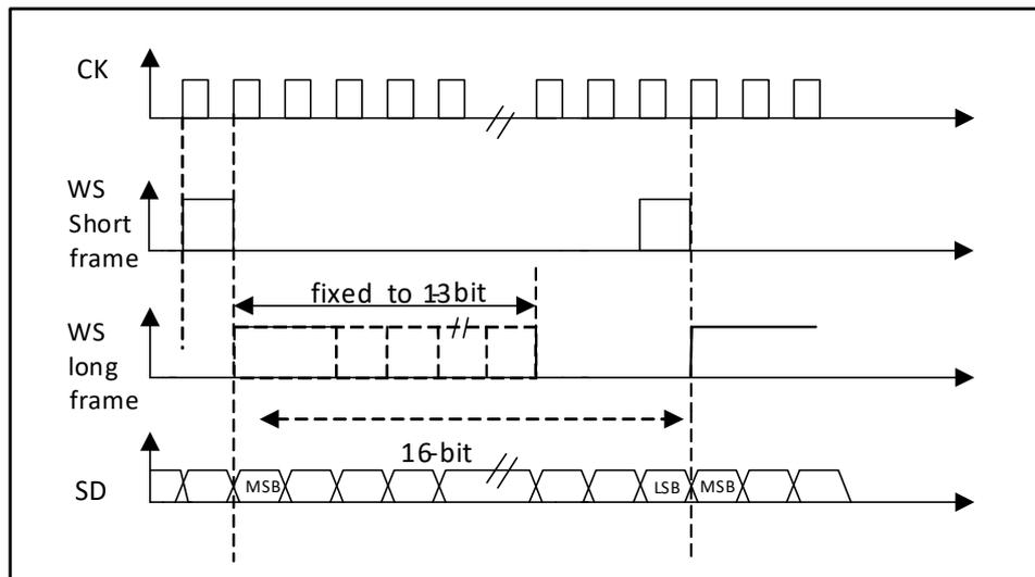
For the long frame, in the main mode, the valid time of the WS signal used for synchronization is fixed to 13 bits. For short frames, the length of the WS signal used for synchronization is only 1 bit.
