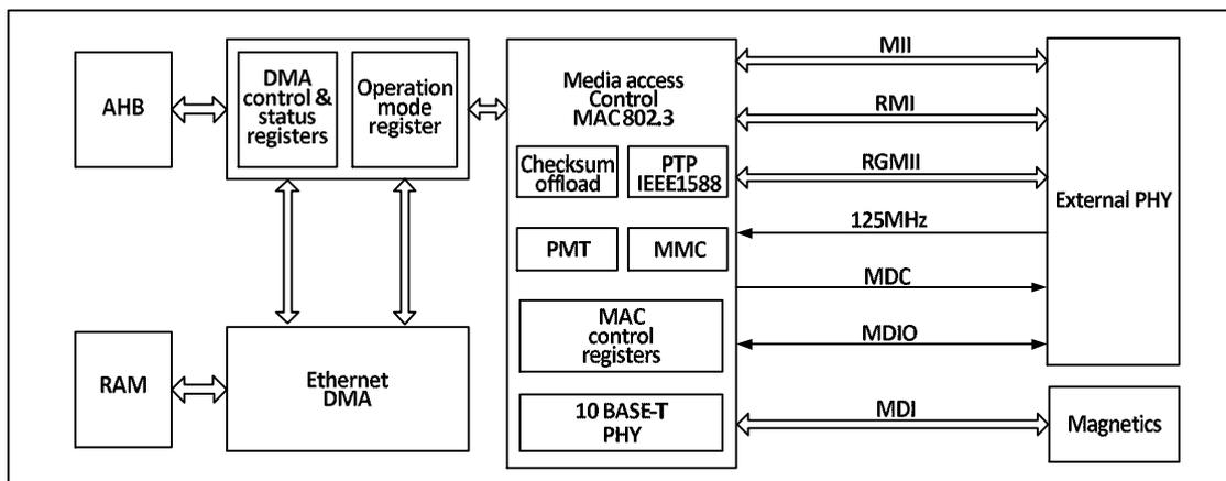
In addition, the Ethernet transceiver also supports the IEEE1588 Precision Time Protocol (PTP) to provide precise time data for microcontroller systems or off-chip.
