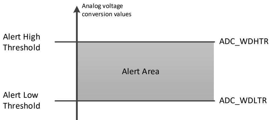
Configure the AWDSGL, AWDEN, JAWDEN and AWDCH[4:0] bits in the ADC\_CTLR1 register to select the channel for analog watchdog vigilance. The specific relationship is shown in the following table:
