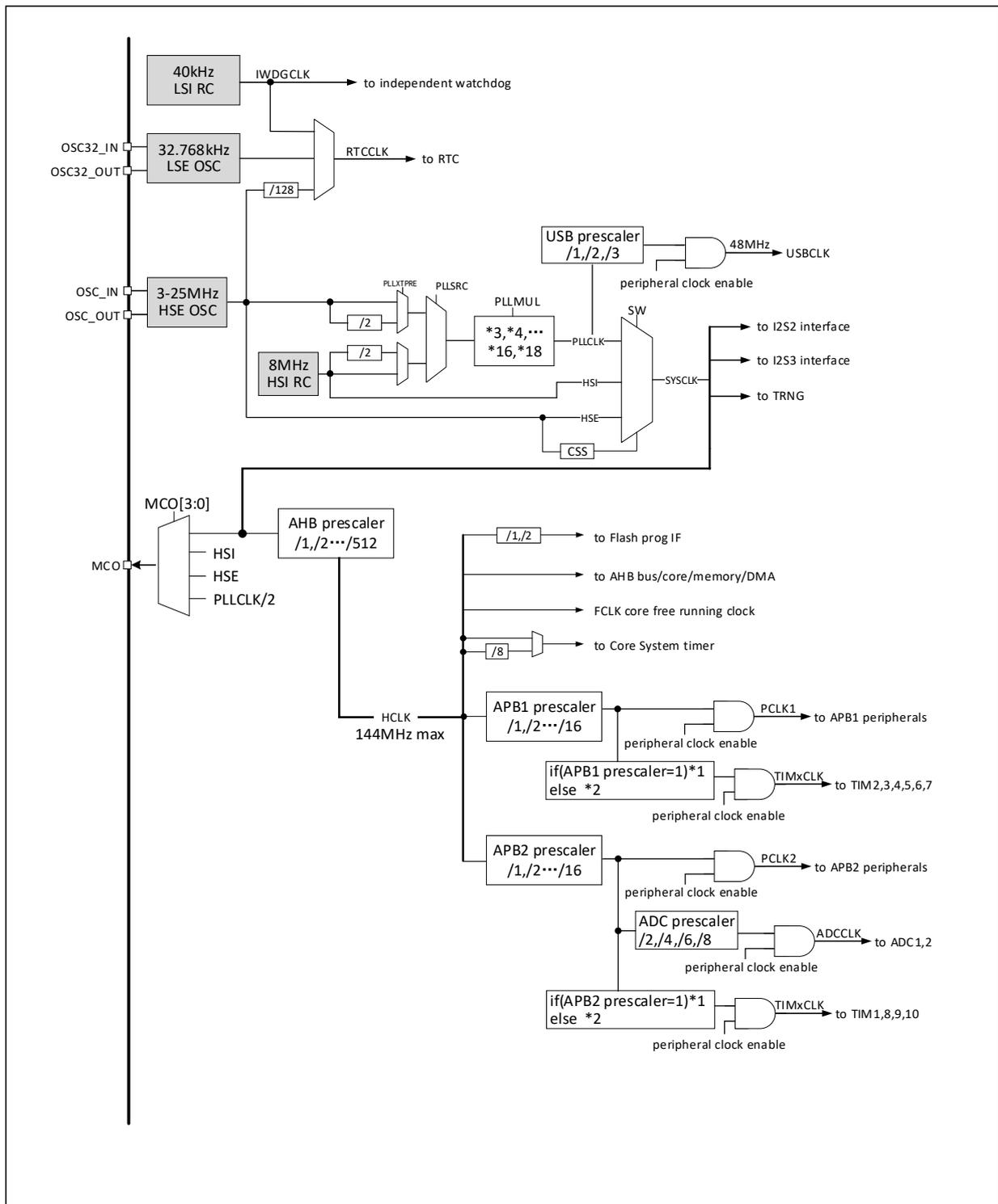
Note: This clock tree structure is applied for CH32F20x\_D6, CH32F20x\_D8, CH32V20x\_D6 and CH32V30x\_D8.
