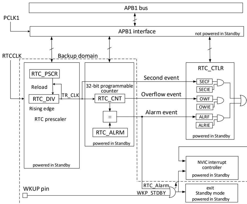
As shown in Figure 6-1, the RTC module is mainly composed of 3 parts: APB1 bus interface, prescaler and counter, control and status registers. The prescaler and counter are in the backup area and are powered by  $V_{BAT}$ . After RTCCLK is input to the prescaler (RTC\_DIV), it is divided into TR\_CLK. It is worth noting that a self-
