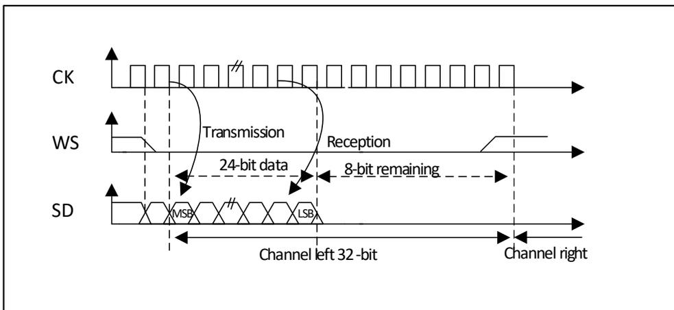
This mode requires 2 read or write operations to the SPI\_Datar register. In transmit mode: if you need to send 0x8EAA33 (24 bits):
