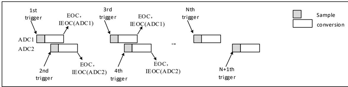
If the injected discontinuous mode is enabled, when the first trigger occurs, the first injected channel in ADC1 is converted. When the second trigger occurs, the first injected channel in ADC2 is converted. And so on. If an interrupt is enabled, an IEOC interrupt is generated after all injected group channels in ADC1 are converted. If an interrupt is enabled, an IEOC interrupt is generated after all injected group channels in ADC2 are converted.
