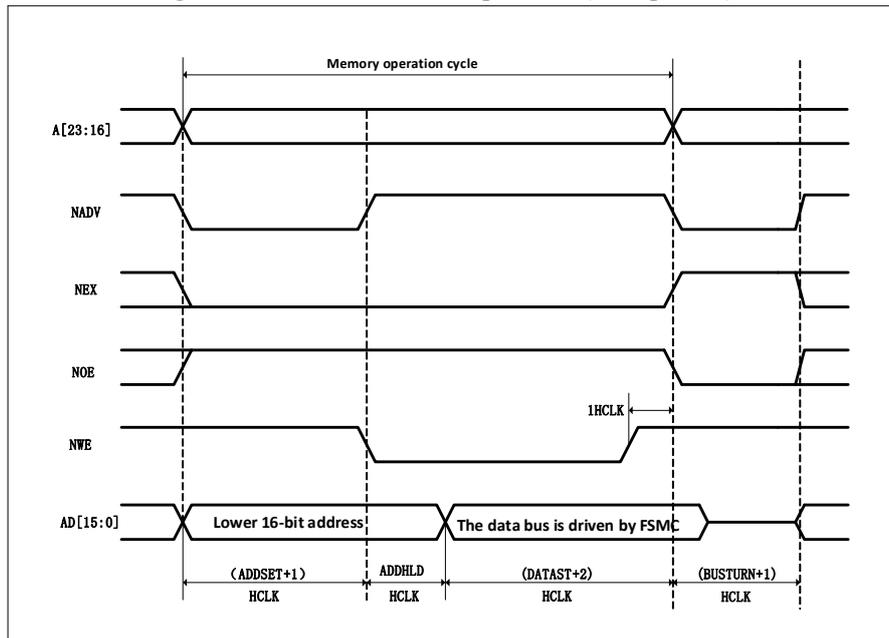
Figure 26-19 Mode D FSMC\_BCR1 bit field
